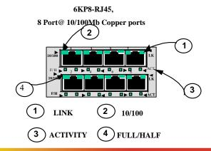
shielded twisted pair (STP) cable connections. The 6KP8-RJ45 module is equipped with a Media Dependent Auto-Crossover (MDI-X) switch, which controls all ports for cascaded connection. This feature eliminates the need for a special twisted pair crossover cable when connecting to a hub or another switch.
